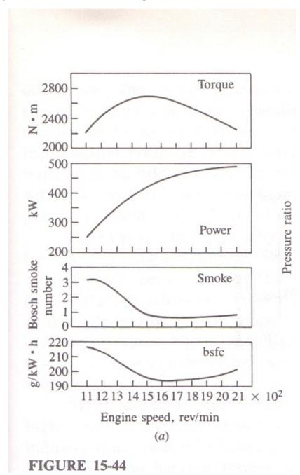
**Fig.15-44:** Performance Characteristics of medium-speed turbocharged after-cooled DI diesel engine. Torque, Power, Smoke number, and bsfc for V twelve-cylinder version. Bore = 128 mm, stroke = 140 mm, rc = 15.
